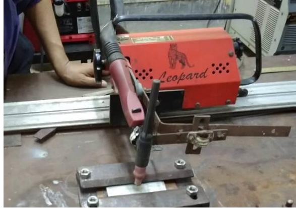
Figure 1 TIG welding set up showing the TIG torch mounted on the vehicle placed on a rail
